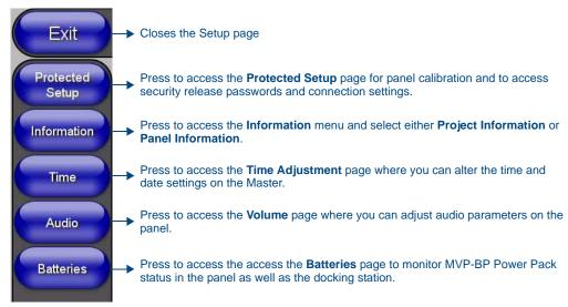
FIG. 45 Setup Page Navigation Buttons (MVP-8400)
